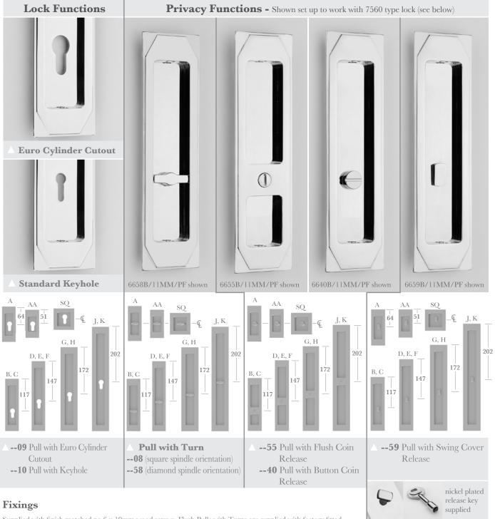
Supplied with finish matched no.6 x 19mm wood screws. Flush Pulls with Turns are supplied with factory fitted 5mm spindles suitable for doors up to 45mm thick if the face plate is surface mounted (or 51mm thick if flush fitted). Longer spindles are available upon request for doors up to 80mm thick.
